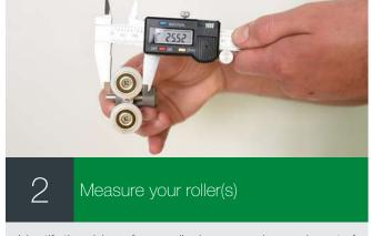
Identify the sizing of your roller by measuring each part of the roller. Bear in mind that some measurements might be 1mm-2mm off due to wear and tear. See below our Roller Sizing Guide.
